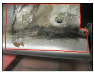
Figure 3 - fender removed (corrosion on the contact surface of the rocker panel [side member])
