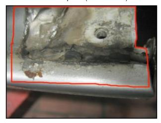
Figure 5 (corroded contact outer rocker panel [side member])
