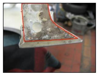
Figure 4 (corroded contact surface of fender)
