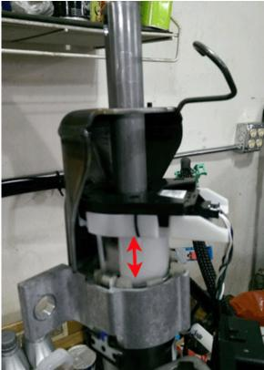
2. The upper intermediate steering shaft to lower column shaft bolt and nut (2) may be contacting the inhibitor/shiftier cable bracket, as shown below.
