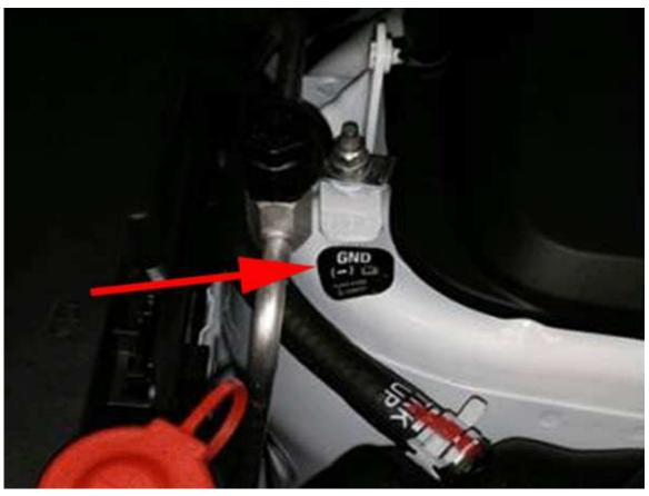
4. After fuse is replaced, install an electrical ground point label, GM P/N 10384767, in the approximate location as illustrated above.
