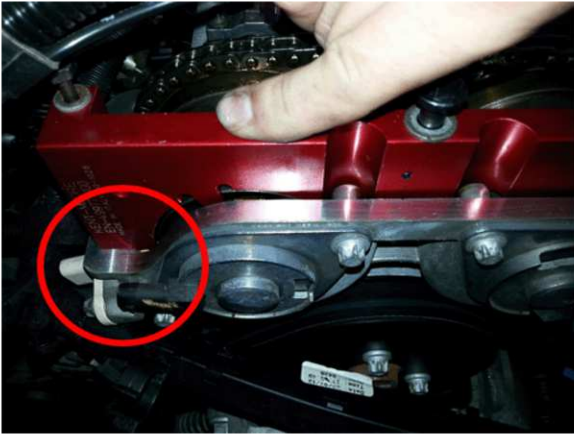
Front Cylinder Head with Tool Showing Exciter Wheel Misalignment
