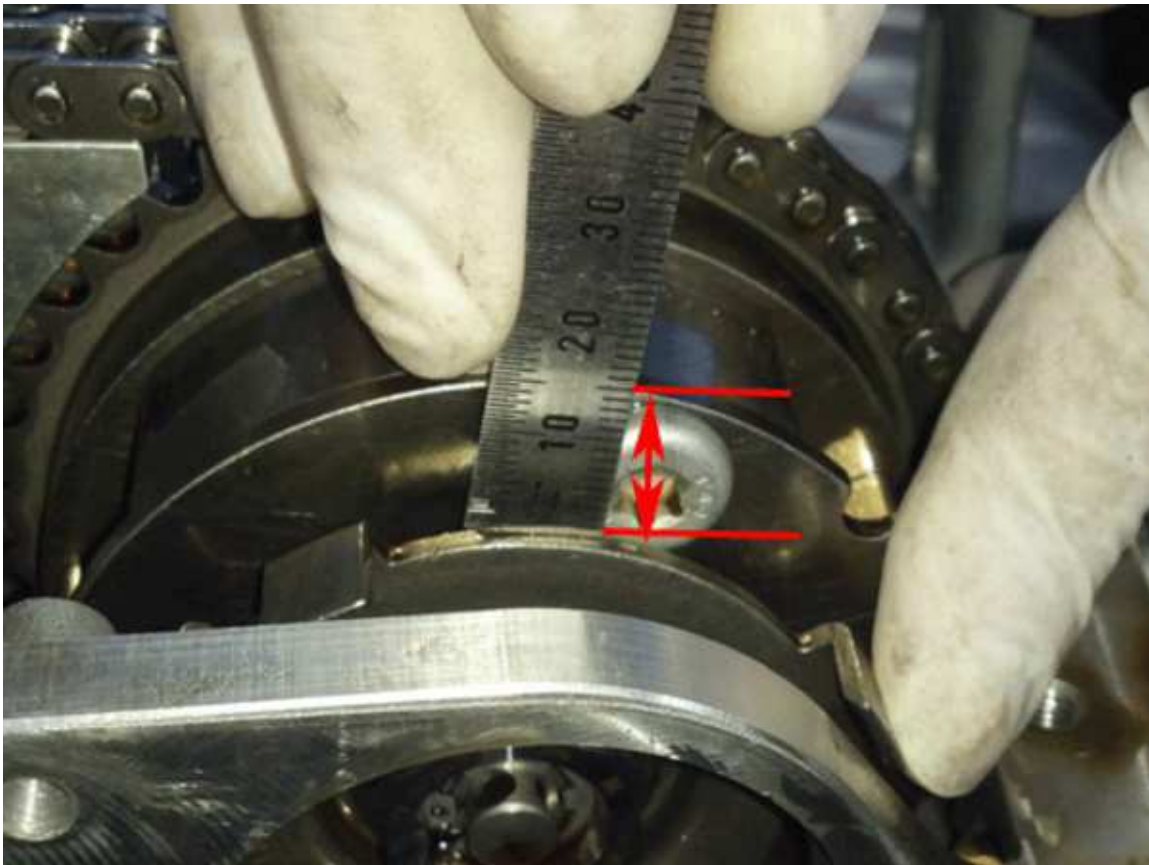
Exhaust Exciter Wheel Correct Alignment
