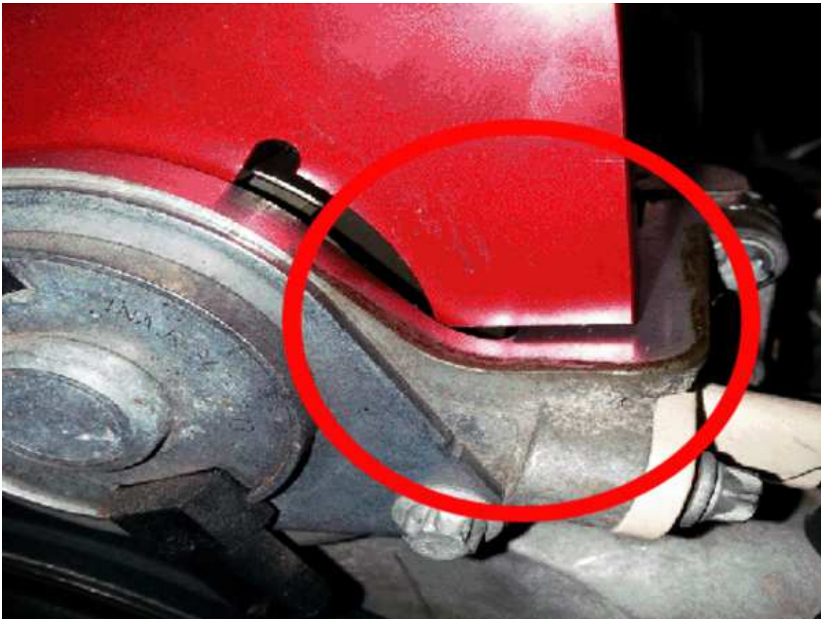
Exhaust Exciter Wheel Incorrect Alignment
