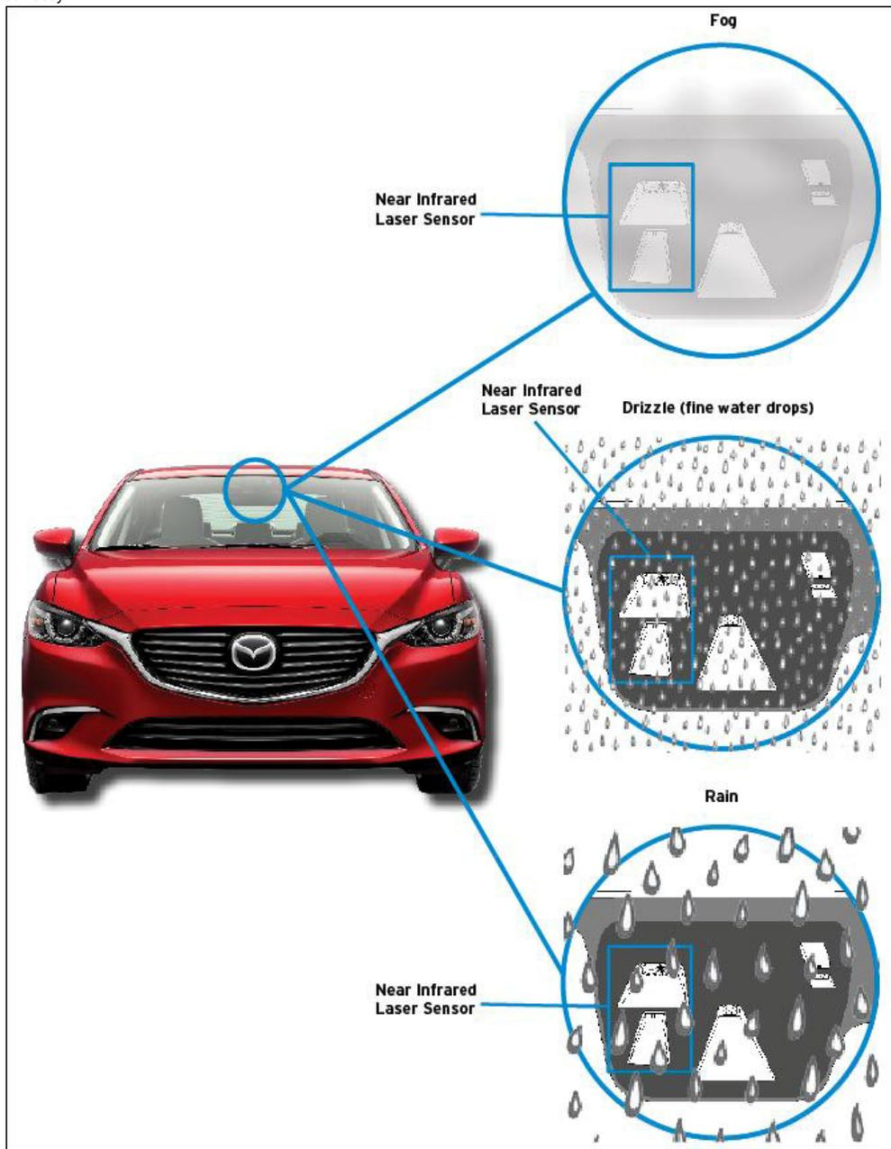
The near infrared laser beam (SENDING) emitted from the laser sensor (SENDER) is refracted by water drop on the windshield and reflects an object (a traffic sign in the figure) outside the normal sending range. The reflected beam (RECEIVING) by the traffic sign is also refracted by water drop and received by the laser sensor (RECEIVER). Thus, the system may detect an object outside the normal detection range as a vehicle and the SCBS operates unintentionally.
