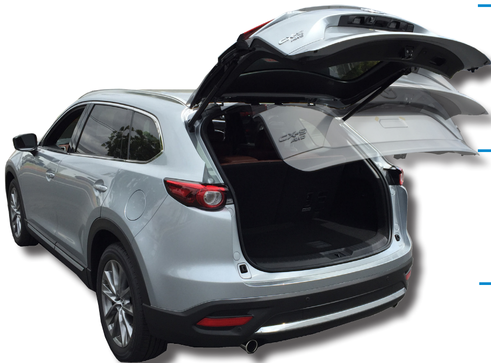
Top half of PLG travel is adjustable
