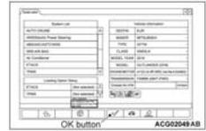
2. When you activate "TPMS" in "Loading Option Setup", you can select "w/o KOS (Can see P/N)" or "w/o KOS (Cannot see P/N)." If the laser marking is visible, select "w/o KOS (Can see P/N)." If not, select "w/o KOS (Cannot see P/N)."
