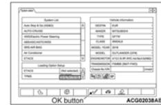
2. When you activate "ETACS" in "Loading Option Setup", you can select "Can see P/N on ECU body" or "Can't see P/N on ECU body." If the laser marking is visible, select "Can see P/N on ECU body." If not, select "Can't see P/N on ECU body."
