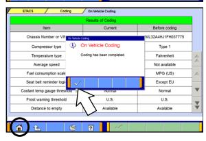
8. Make sure the coding file is highlighted (contains ETACS ECU P/N and vehicle VIN), then click the check mark at the bottom of the screen.
