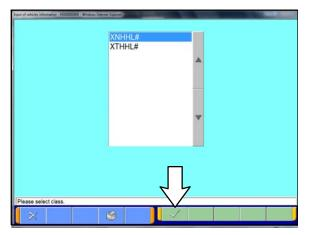
d. Click the icon in the lower RH corner of the screen to have MUT–III automatically read the VIN.
