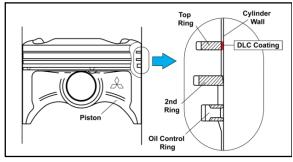
b. Top piston ring contact surface has Diamond Like Carbon (DLC) coating to reduce friction.
