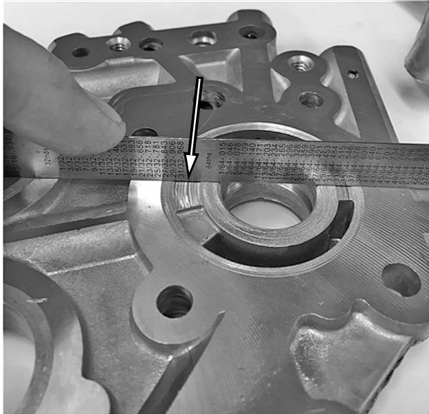
Figure 6. Measure Plate Wear
