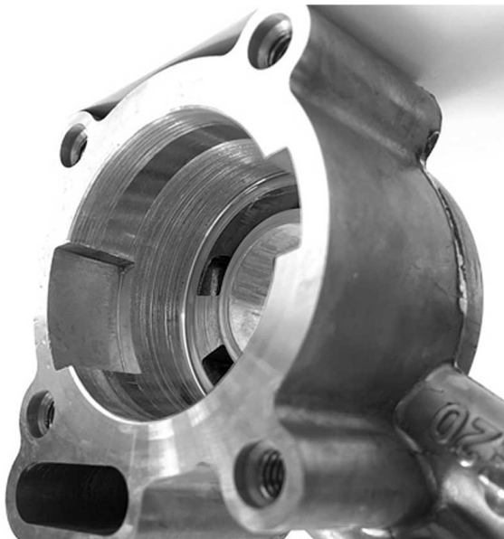
Figure 8. Excessive Housing Wear
