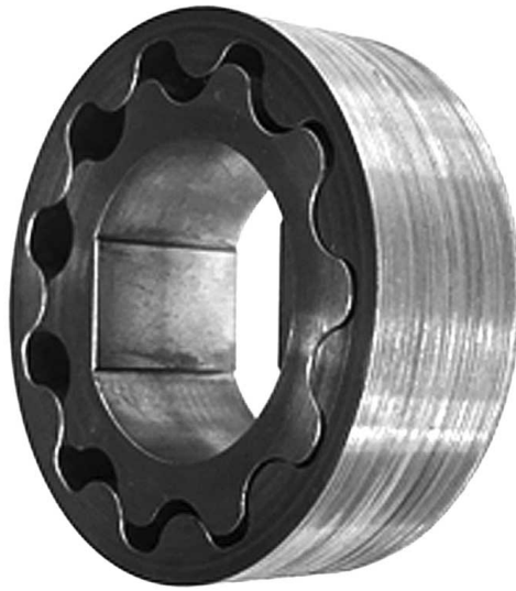
Figure 3. Wear that is less critical to pump performance. Measurement is required. Inspect the housings and plates:
