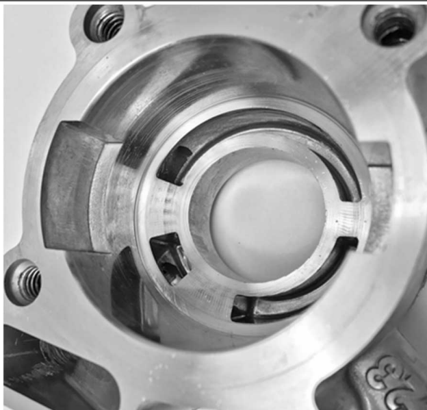
Figure 7. Typical Housing Wear
