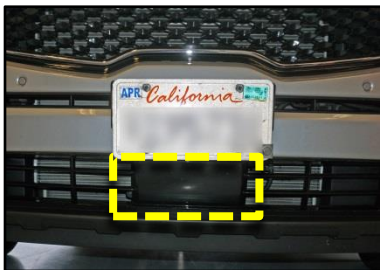
Radar module unobstructed; plate mounted correctly
