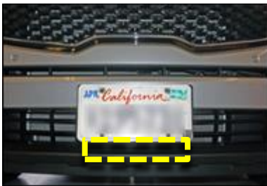
Radar module partially blocked; plate mounted incorrectly
