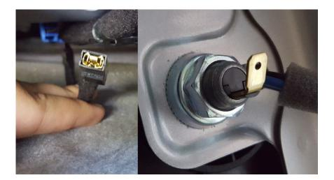
Disconnect connector B and use a small brush to apply Stabilant 22A to the Main To Antenna Harness Connection AM/FM input pin (Pin 2). Note: Allow five (5) minutes of drying time after applying Stabilant 22A, prior to reconnecting the connector.
