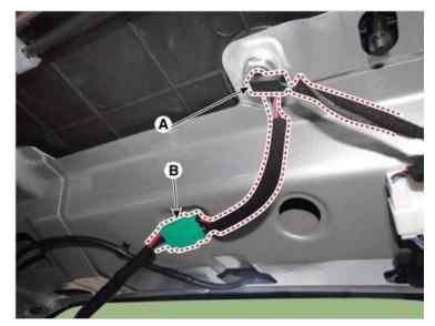
3. Ensure the power connector at the base of the antenna (A) is seated properly and check terminal tension.
