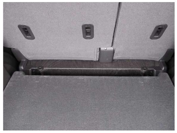
Starting with 2014 vehicle production, the floor filler trim panel was eliminated as standard equipment. The seat/floor interface will now look like the example shown in the graphic above.
