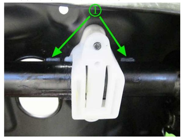
Important: On some vehicle models, a production change added welded brackets (1) to the seat crossbar on each side of the guide block to help retain its position. On these particular vehicles, it will be necessary to rework the new clip service part to ensure proper installation to the crossbar.
