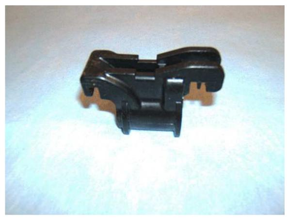
A clip has been made available to eliminate the lateral seat movement. Use the following steps to install the clip to the driver side seat. If the vehicle is equippec with a 6-way adjustable passenger seat, repeat the procedure on the passenger seat.
