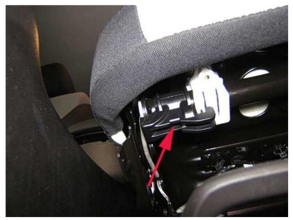
3. Install the clip as shown. Ensure the clip is fully seated around the crossbar and on the guide block.
