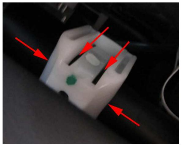
**Note:** Spray Super Lube, P/N 12346241 (in Canada, P/N 10953474), or equivalent to the areas on the white clip, as shown in the illustration above, to ensure that the noise is eliminated.
