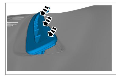
Note! Avoid spillage on visible surfaces. Install the marked component.
