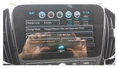
If the customer wants to select delayed or rate based charging when he is outside the home location, the customer will have to turn off the location based charging for the options to be selectable again. This is done through vehicle personalization in the center stack by selecting: Home Screen/Settings/Vehicle/Energy/Location Based charging
