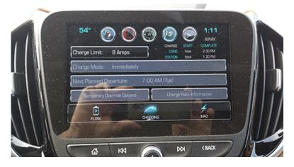
**Note:** The only option available for "Away" mode is immediate charging. This is made as a convenience for the customer so they do not have to initiate an immediate charge when they are at a routinely visited charging location away from home.
