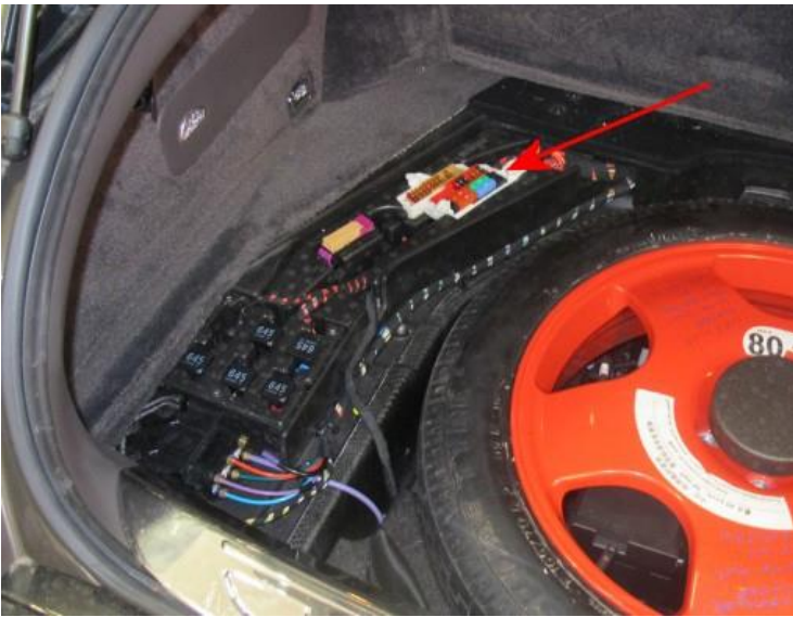
Figure 3. Remove fuse 1 - 40A - Adaptive Suspension Compressor Relay - figure 4.
