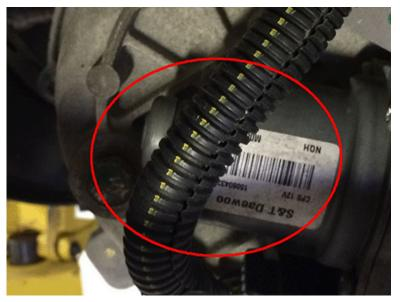
Concerns in the area near the encoder motor on the transfer case may cause: Various IPC warning lights to illuminate.
