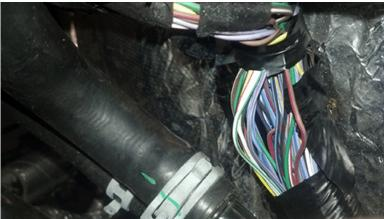
Concerns in the area of the coolant pipe / clamp / clamp tabs between engine and cowl may cause: Various IPC warning lights to illuminate. The Service Four Wheel Drive (4WD) light may illuminate. The Stabilitrak light may illuminate. The check engine light to illuminate. DTCs associated with chafing in the area may include: B1011, P0575, U0073, U0100, U0121, U0140, U0415 and U0420.
