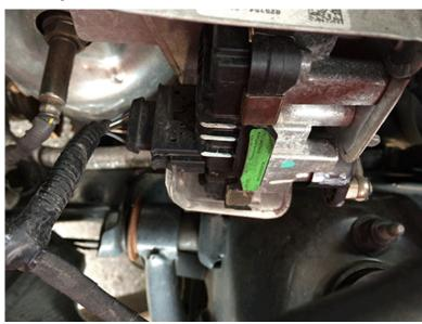
Concerns with loose terminals or connector not fully seated at the Turbocharger Vane Position Actuator may cause:
