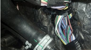
Concerns in the area of the coolant pipe / clamp / clamp tabs between engine and cowl may cause:
