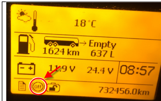
FIGURE 41 : PRIOR UNDERTAKING THIS PROCEDURE, (OFF) PICTOGRAM DISPLAYED ON THE DID STATUS LINE
