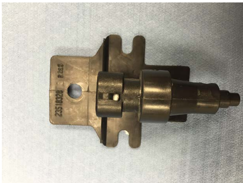
Figure 2 – Correct Ambient Air Temperature Sensor P/N: 23518328
