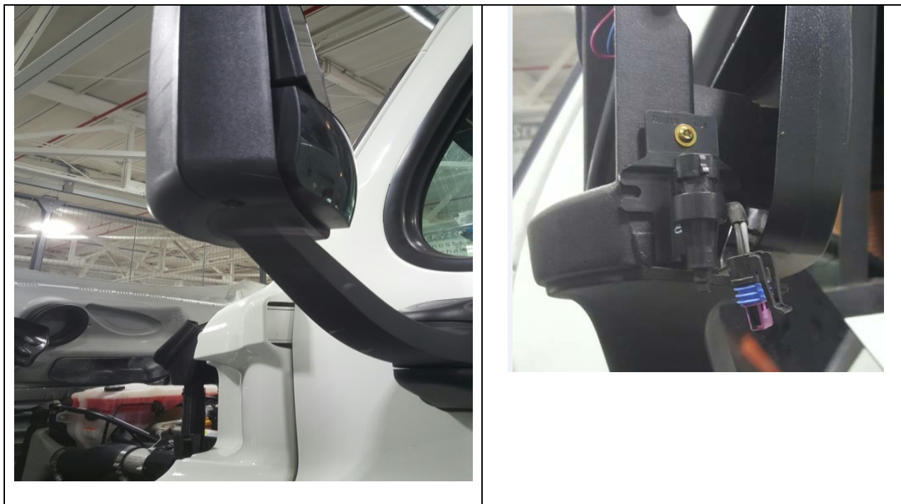
Figure 3 – Sensor Location in Cascadia and Coronado Chassis
