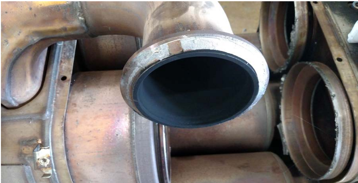
Figure 1 – Original DOC Inlet Flange
