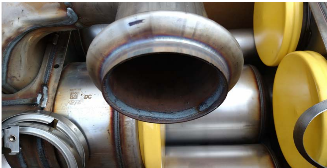
Figure 2 - New DOC Inlet Flange
