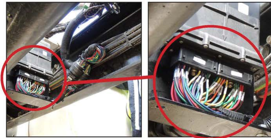
Figure 13: Straighten the harness wires from the connector node and then bend at a 90° angle on the bracket.
