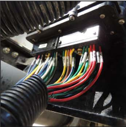
Figure 11: Connect the jumper harness connectors to the McNeilus Command Center node.
