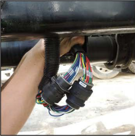
Figure 10: Connect the jumper harness Deutsch connectors to the chassis harness.
