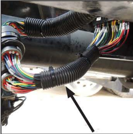
Figure 12: Install the black harness cover with zip ties.
