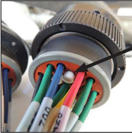
Figure 8: Insert blank pin plugs into unused pin positions.
