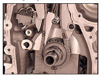
4. The procedure for installing the wedge tool in the latest version of 06-06-01-017 advises that the wedge should be lightly seated using a couple of very light taps with a small plastic or brass hammer
