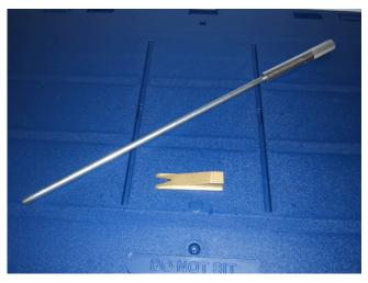
If the tool handle unscrews from the threaded rod, leaving the threaded rod screwed into the wedge as shown below, apply thread locker to the threads of the tool handle and screw it onto the threaded rod to prevent it from coming off in the future.
