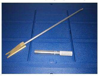
3. When inserting the wedge, ensure that it is installed in the correct direction as shown below.
