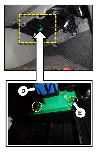
6. Replace the blower motor and the resistor.
