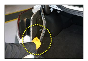
3. Use a non-marring trim panel tool to remove the trunk garnish plastic rivets.
