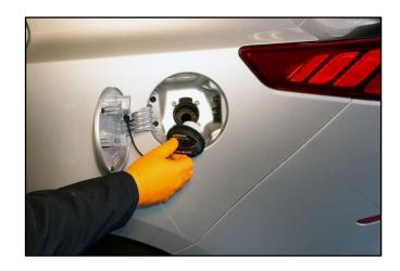
6. Use a 10mm socket to remove two (2) bolts securing fuel door actuator trim bracket.
