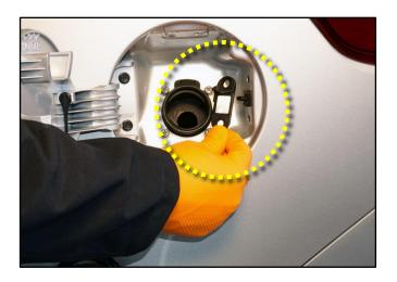
8. Remove wire harness connector from the fuel door actuator.
