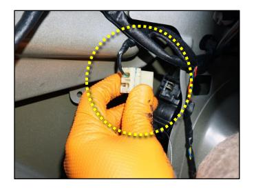
9. Remove the fuel door actuator assembly from the vehicle.
