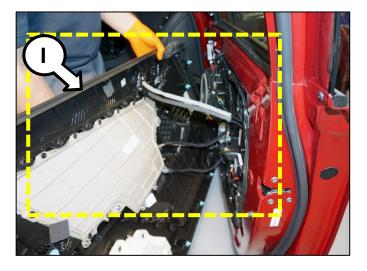
11. Remove four (4) screws (J) securing the speaker (K) to the door module.
