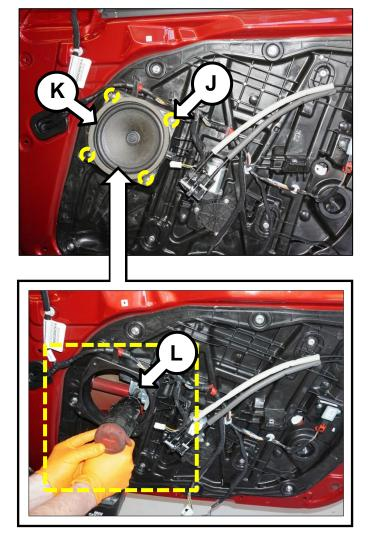
12. Remove one (1) bolt (L) securing the door glass in place.
