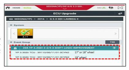
If the ROM ID is not correct, reference the ROM ID information table (see below), the PCM/TCM can be corrected by performing another **Manual Mode** reflash. However, please ensure the correct PCM/TCM part number is selected to prevent any further drivability concerns and verify that the correct ROM ID is loaded after the reflash has been completed.
