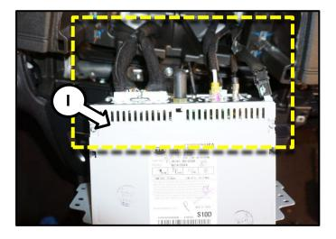
10. Install the replacement head unit, and all other removed components, by reversing the order of removal.
