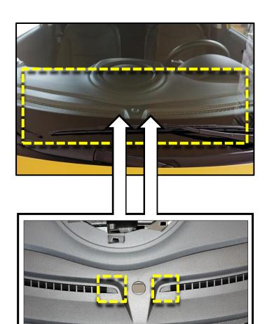
3. Apply downward pressure on each vent clip to secure in place, as shown.
