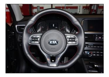
4. Turn the steering wheel 90° to the left and insert a small screwdriver from behind the steering wheel, as shown, to undo the tab (B) securing the airbag module.
