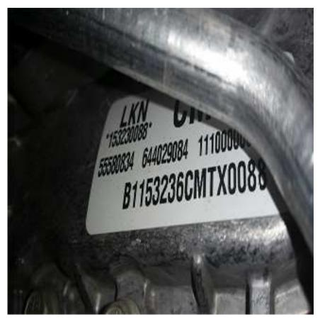
As shown in the above photo, the engine broadcast code can be found on the engine front cover.
