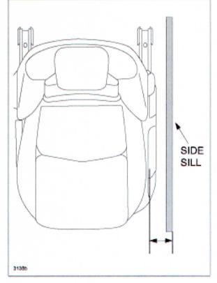
When you receive a customer complaint for this concern, explain that the seat may move down by leg touching the seat adjustment lever when getting in or out of the vehicle. Confirm that the seat position is appropriate before driving.
