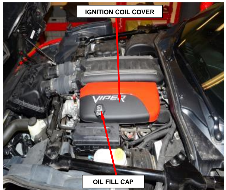
Figure 2 – Ignition Coil Cover
