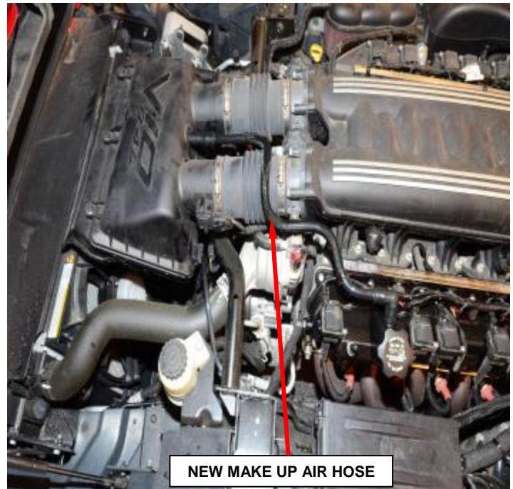
Figure 7 – New Make Up Air Hose
