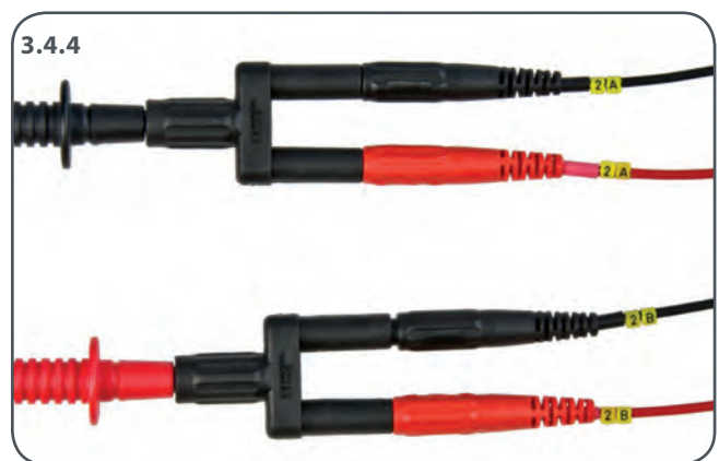
3.4.4 When using several test leads, always ensure that the leads marked A and B are correctly assigned.
