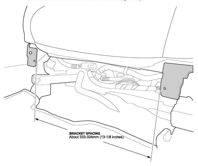
4. Adjust the distance between the seat bracket and center console with a pry bar. Once the bracket measures about 333–334mm (13-1/8 inches) go to step 6.
