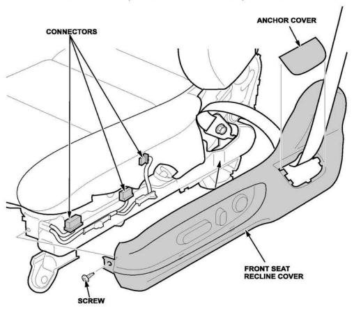
Adjust the seat to the rear position and remove the seat belt anchor bolt.
