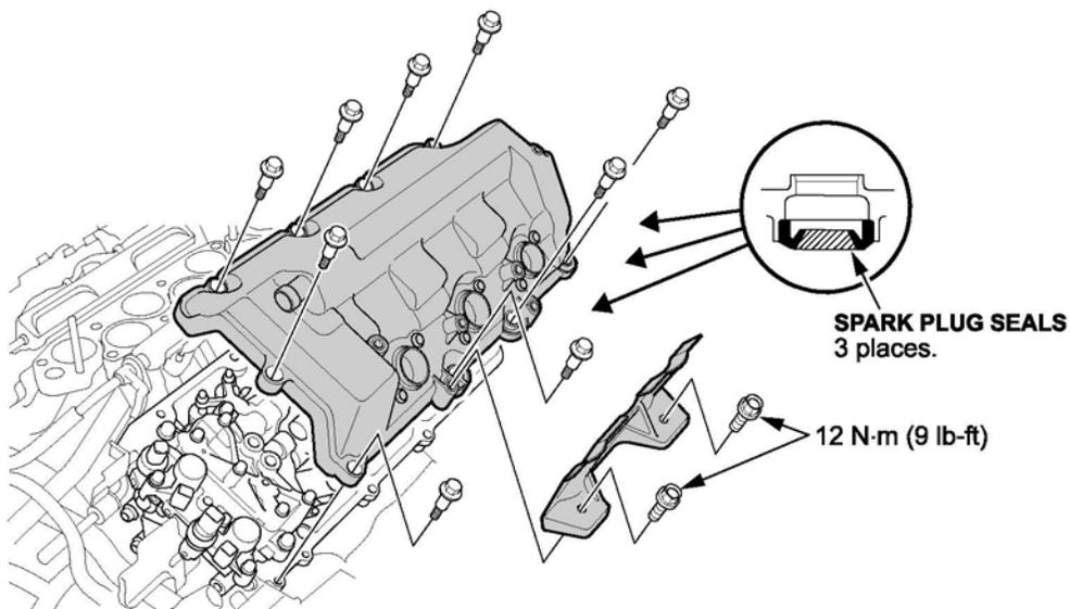
9. Inspect the plug seals for any damage.
