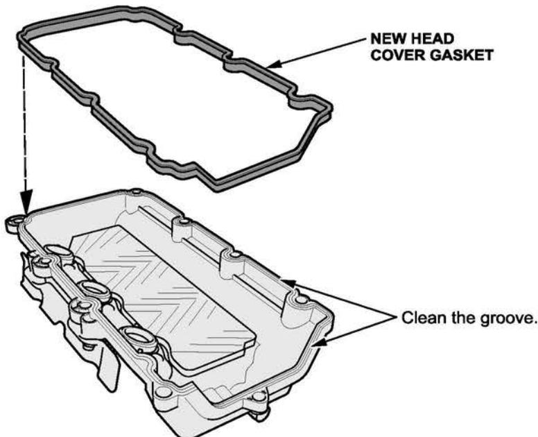
7. Apply liquid gasket on the chain case and the No. 5 rocker shaft holder mating surfaces. Then, install the head cover within 5 minutes of applying the liquid gasket.
