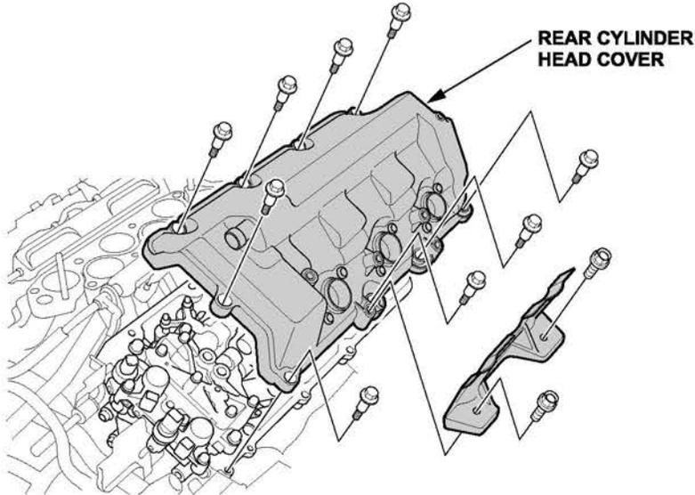
4. Remove the head cover gasket from the rear cylinder head cover.
