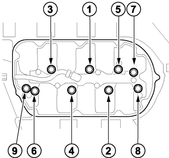
12. Install the intake manifold upper cover and torque the bolts and nuts in three steps to **12 N·m (9 lb-ft)**.
