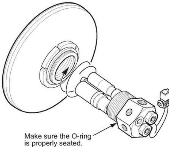
4. Position the 2.5-Inch socket over the solenoid valve with the pigtail harness coiled up on the end of the valve to fit it into the socket.
