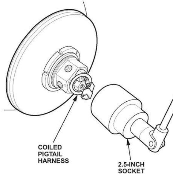
8. Use the breaker bar supplied in the kit to loosen the solenoid valve.
