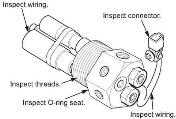
2. Connect the solenoid valve test harness from the kit to the solenoid valve 2-pin connector.
