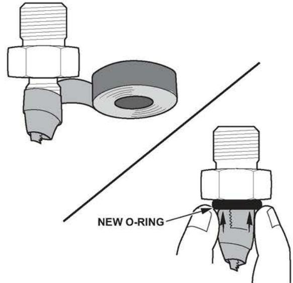
9. Install the three different connectors finger-tight in the correct port.
