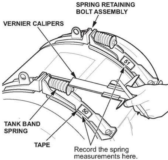
2. Measure both of the tank band spring lengths using a Vernier caliper. Record the measurement on the piece of tape that was placed on the tank band. You will need this later for reassembly.
