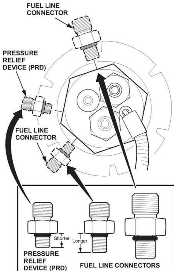
10. Install the three main fuel line connectors by making sure the tank is on its side, then, using a 5/8 inch crowfoot wrench on the smaller fittings and a deep socket on the large fitting, torque the fittings to:
