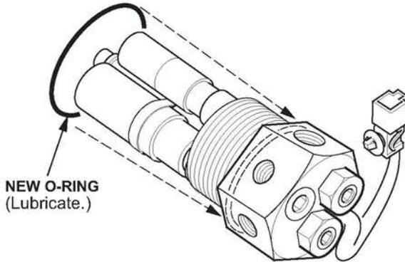
3. Hand thread the solenoid valve into the tank making sure the O-ring seats properly into its groove.
