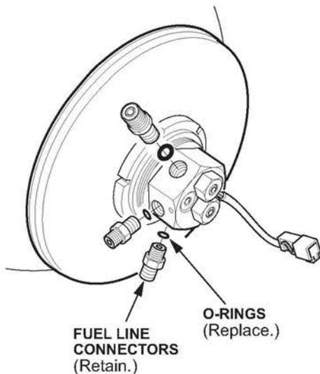
6. Note the position of the line connectors. Remove the three fuel line connectors.
