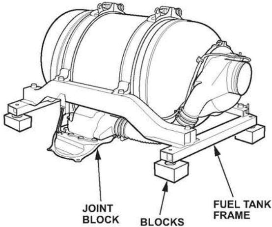
3. Use the large plastic wire tie to support the fuel joint block lines up to the frame. Make sure that the joint block bracket is attached. Leave the wire tie in place until the lines are reattached to the new solenoid valve.
