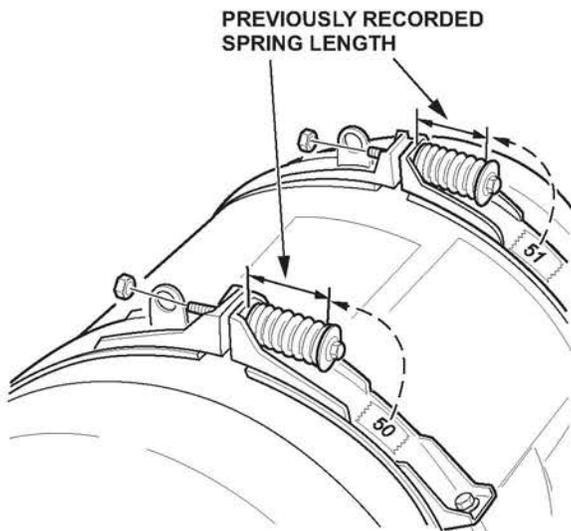
9. Make sure the vertical lines on the tank align with the tank bands.
