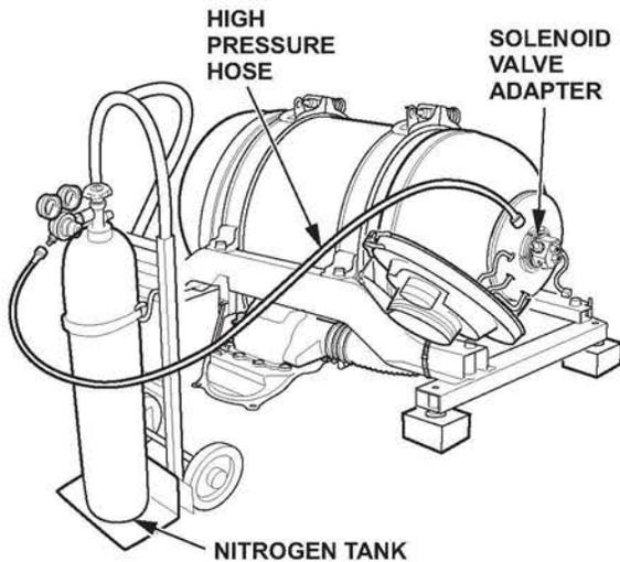
4. Open the main nitrogen cylinder valve number 1:
