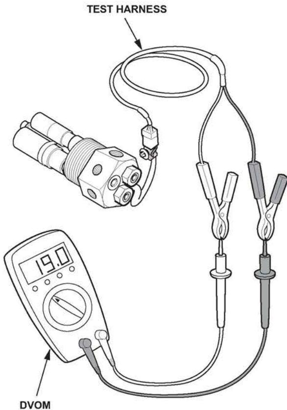
4. Momentarily connect the test harness to an automobile battery or booster pack, and electrically activate the solenoid valve.
