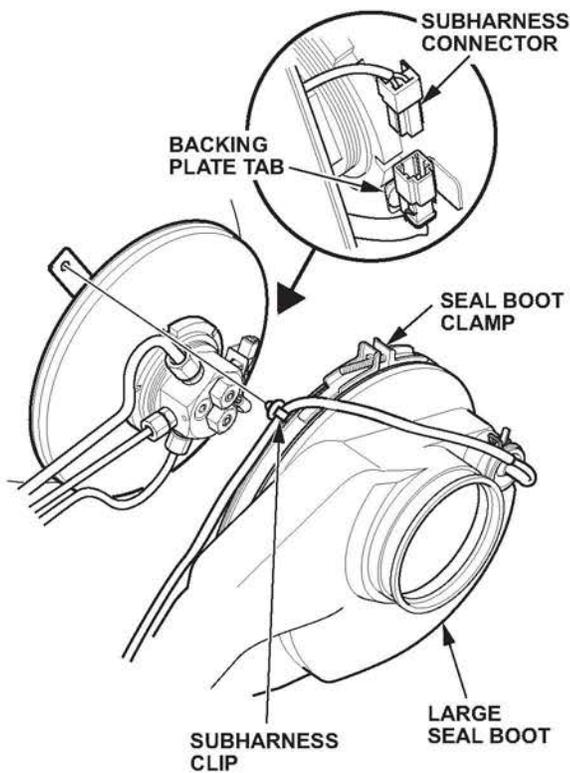
4. Connect the 2-pin solenoid sub harness connector to the wire harness on the tab.
