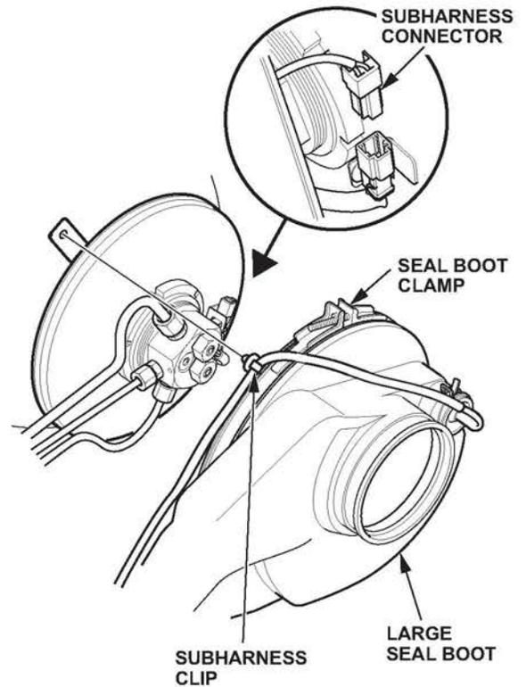
2. Fold back the seal boot to access the fuel lines.
