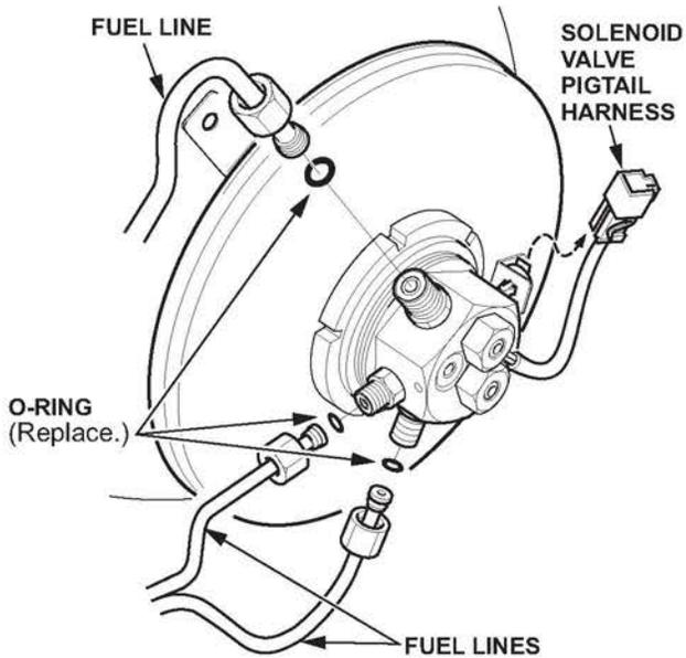
4. Disconnect the solenoid valve pigtail harness from the backing plate clip.
