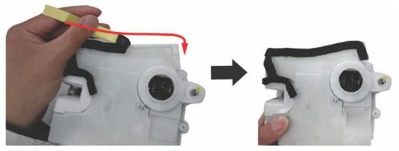
5. Apply the connector seal to the door latch assembly as shown.
