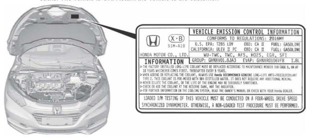
2. Inspect the emission label to make sure 2016 is the model year listed as shown.
