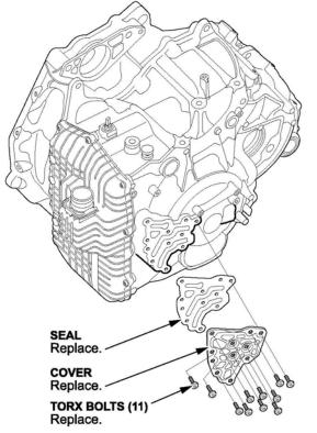
7. Replace the cover, the sealing gasket, and bolts with the new ones from the kit. Torque the bolts to **10.0** N·m (7 lb-ft) in the sequence shown.
