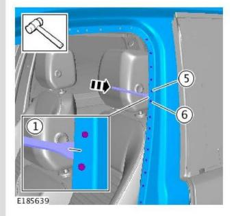
Insert the chisel to a maximum of 10mm (1).
