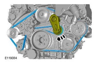
3Remove the accessory drive belt idler pulley cap.
