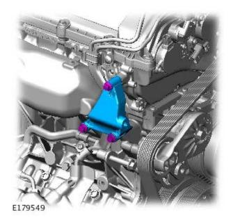
5Install the new accessory drive belt pulley bracket.
