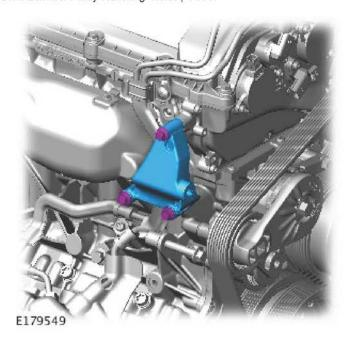
**5**Install the new primary drive belt pulley bracket.
