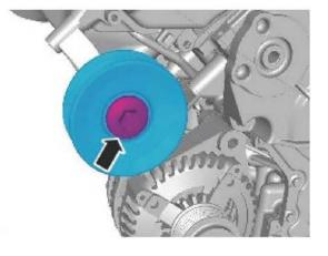
**4**Remove the primary drive belt idler pulley bracket.
