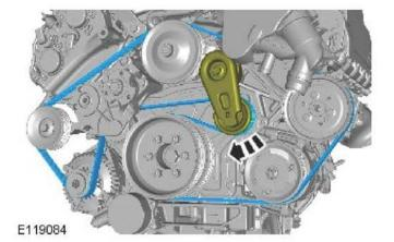
3Remove the primary drive belt idler pulley cap.
