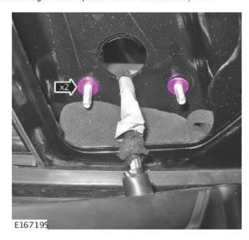
**5**Install the powerfold door mirror.
