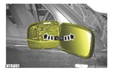
2 NOTE: do not disconnect the powerfold door mirror - trim electrical connector.
