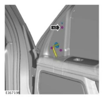
**4**Install the washers to the powerfold door mirror lower retaining bolts only.
