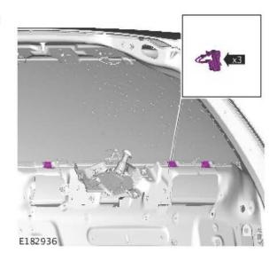
NOTE: the tailgate trim panel clips must be installed into the tailgate in the order shown.
