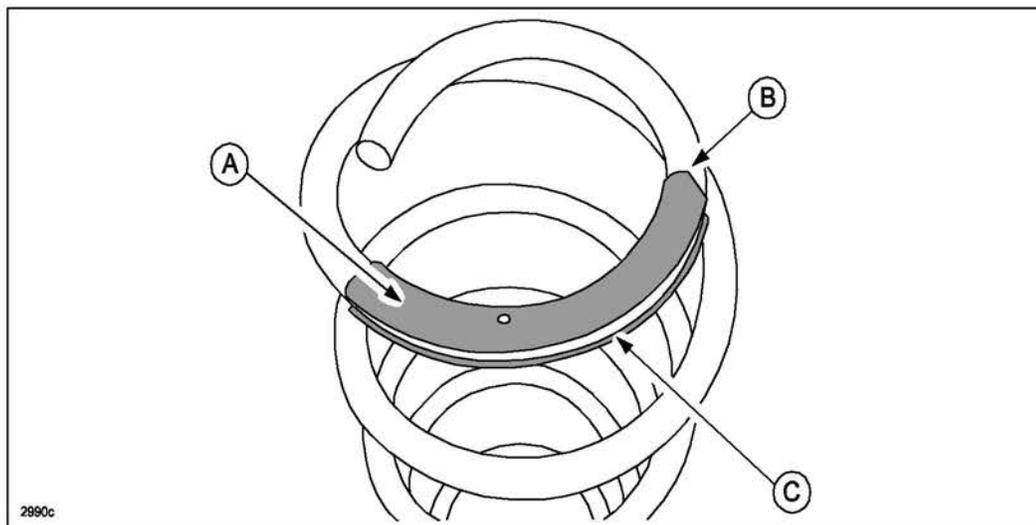
11. The inner side of the protector contains adhesive glue. After installing the protector onto the spring, press the inner side to firmly adhere it to the spring.
