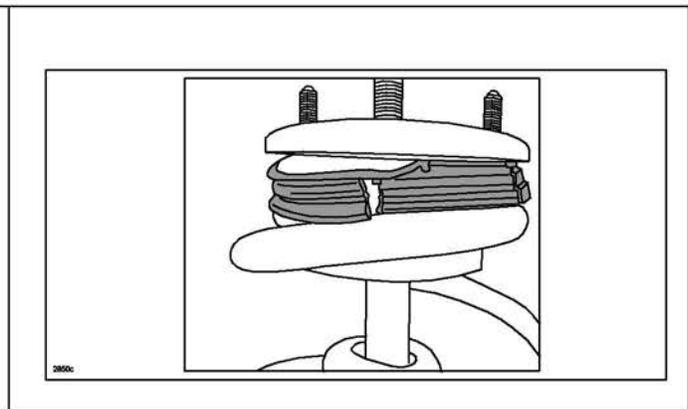
3. Install a protector on the front coil spring. Refer to "PROTECTOR INSTALLATION PROCEDURE" in page 5.
