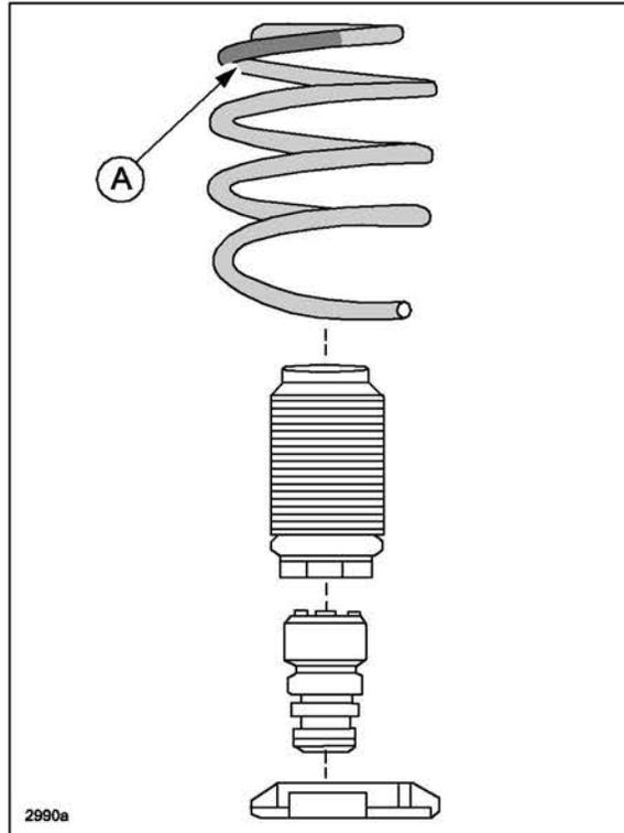
6. Starting from the top of the coil spring, degrease the spring 1.5 coils downward.
