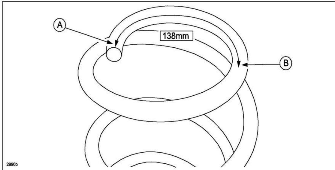
10. Install the protector (A) onto the coil spring aligning the end (slant cut side) with the marking at spot (B).
