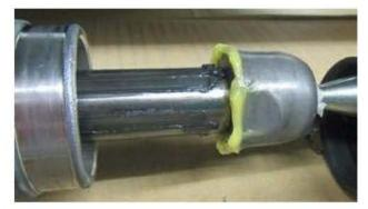
11. Reinstall the boot using a new boot band.
