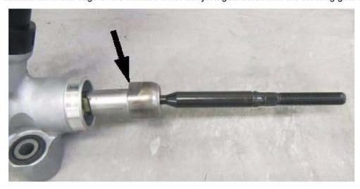
To eliminate the noise, the shape of the inner ball joint edge has been changed.
