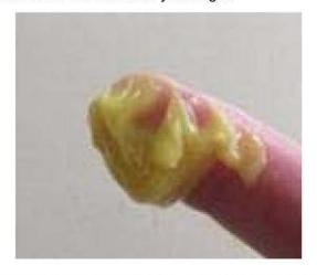
10. Apply the grease all the way around the inner ball joint edge (as shown below).
