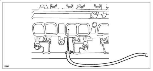
c. Scrape the carbon deposits off of the stems and intake valves using shop towels and an appropriate plastic or wooden stick.
