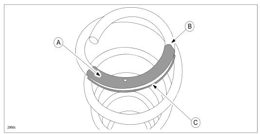
f. The inner side of the protector contains adhesive glue. After installing the protector onto the spring, press the inner side to firmly adhere it to the spring.
